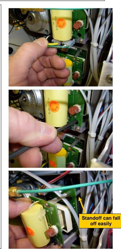
Carefully wiggle out and remove the six pin connector along the top edge of the board. Note that it connects to the leftmost six pins on the board before removing it. Also note the orientation ( brown wire on right side ).
