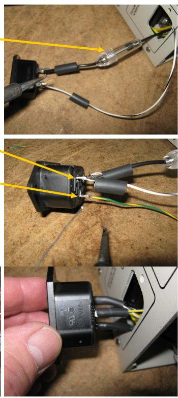
Crimp the two green/yellow wires (from solid state relay and from power jack) to a single ring terminal and then connect the ring terminal to the chassis ground stud with a lockwasher.
