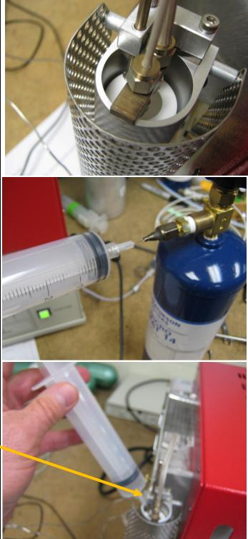
As you push the calibration gas into the vial you should see the vial pressure increase.
