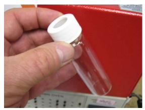
A headspace vial like the 40ml vial shown above is half filled (20ml) with liquid and then the gas above the liquid is purged with inert gas like argon, nitrogen or helium. Gases (CH4, CO, CO2 etc) which are dissolved in the liquid then escape into the inert headspace where they accumulate until an equilibrium is reached. Those gases are then injected into the GC.
