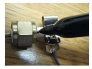
It's a good idea to make a magic maker line on the alumina before removing.
