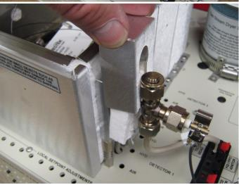
Remove the insulation carefully to avoid breaking off any.
