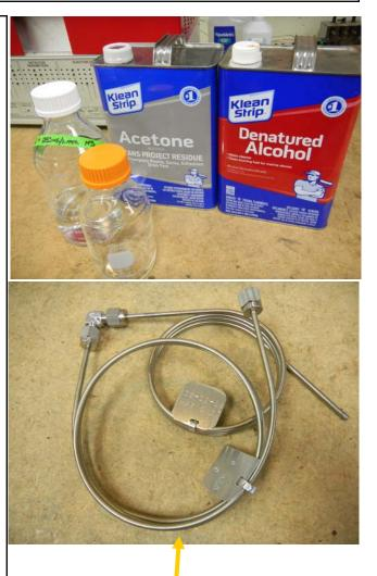
The combo column consisting of a 3 foot Haysep-D and a 3 foot Haysep-R connected in series with a stainless steel fitting can be ordered using SRI part#8600-3D3R which has a list price of \$390 as of January 2017
