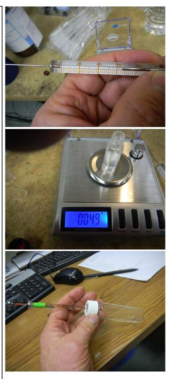
Place the 40ml vial into the incubator for a few minutes to make sure the 1ul liquid calibration standard is completely evaporated in the 40ml vial.
