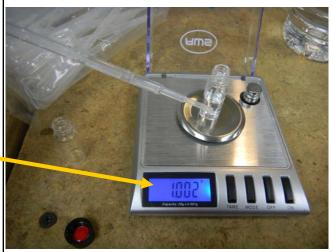
Using the 100ul syringe supplied with the SRI GC, measure 64ul of pure ethanol and add it to the 1ml of water.
