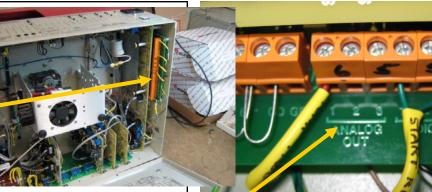
The A/D board is labeled Analog Out 1,2 and 3 if your A/D board is a model 302 6 channel USB type.
