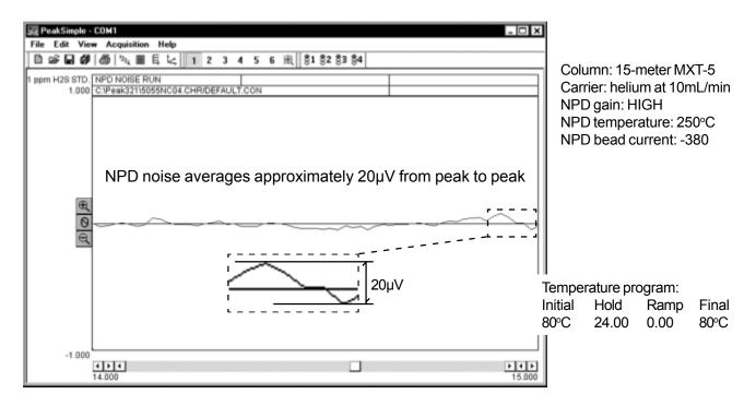
*Note:* Most SRI NPDs are installed on a GC with one or more other detectors. Therefore, SRI tests its NPD detectors with helium carrier gas.
