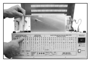
3. Set the NPD detector temperature to 250°C: hold down the SETPOINT button while turning the detector heat trimpot until the desired setpoint is visible in the LED display.
