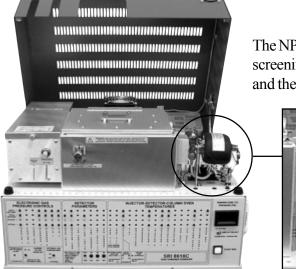
The NPD may be combined with the DELCD for pesticide screening. The NPD detects Organo-phosphate pesticides and the DELCD detects the chlorinated pesticides.
