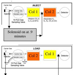
Column 1 is a 3' Haysep D and Column 2 is a 6' MS13X. The Haysep D does not separate Oxygen and Nitrogen or CO. Set the Stop-Flow solenoid time by finding the gap between Methane and CO2, in this case about .9 minutes.
