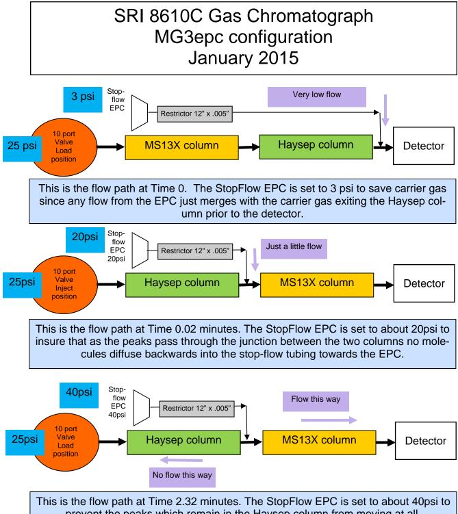
This is the flow path at Time 2.32 minutes. The StopFlow EPC is set to about 40psi to prevent the peaks which remain in the Haysep column from moving at all. The peaks (H2, O2, N2, CH4 and CO) which have already passed into the MS13X column continue to move towards the detector
