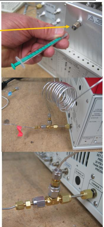
The other end of the restrictor tube is connected to the sample IN port on the front of the valve oven.
