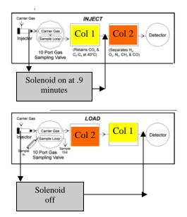
CO migrating onto Column2 (Mole-Sieve13X) where they separate and elute into the TCD detector. Once CO elutes (about 4.00 minutes), the valve is rotated back to the Load position and the Stop-Flow solenoid is de-energized.
