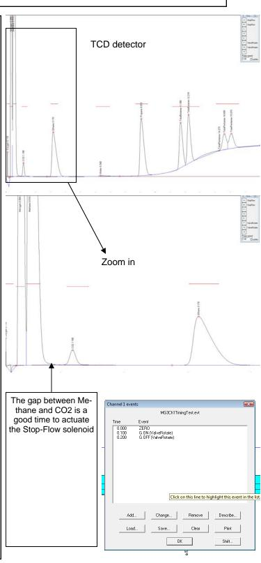
With the Event table modified, the Oxygen, Nitrogen and Methane separate on the MS13X. Then the Stop-Flow solenoid is de-energized and valve rotated back to Load position ( both at 4.00 minutes ) and the remaining peaks ( Ethane, Propane, Water, Butanes, and Pentanes ) which were immobilized on
