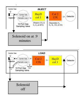
(.1 minutes) the separation occurs as if Column2 was not even connected. (no hardware changes are required to produce this effect). There is a convenient gap between Methane and CO2 where it would make sense to activate the stopflow solenoid valve to immobilize the CO2 and heavier peaks in Column1 while the H2, O2, N2, Methane and CO peaks elute from Column2.
