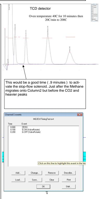
The same sample is injected again using the Event table shown at right. The valve stays in the Load position until 4.00 minutes. The Stop-Flow solenoid is actuated at .9 minutes ( determined from the chromatogram on the previous page ) and de-activated at 4.00 mintes. This results in H2, O2, N2, CH4 and
