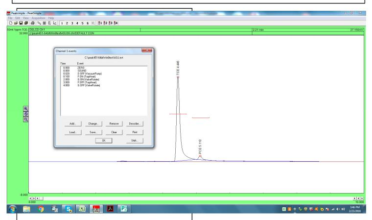
In this chromatogram Relay G was turned off at 4 minutes which allowed the TCE to appear but not ( or mostly not ) the PCE peak. By adjusting the Relay G off time by trial and error you can control which peaks make it onto the analytical column.
