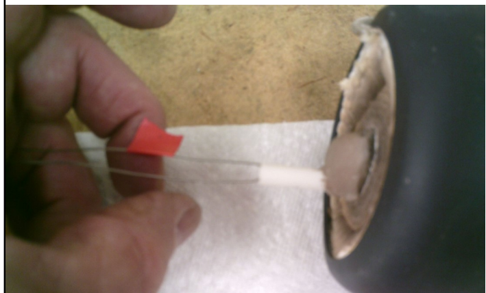
Insert the retaining wire in one end of the tube furnace up to the mark.
