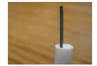
Notice that the blade of the ignitor tilts slightly backward. The tilt positions the tip of the blade just slightly behind and below the tip of the jet. As you tighten the graphite ferrule use the magic marker line to be SURE the ignitor does not twist as you are tightening the nut. If the blade twists against the FID jet the blade may snap.
