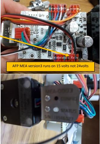
The AFP version 3 MEA also has a serial number etched in the metal bracket making it easy to identify.
