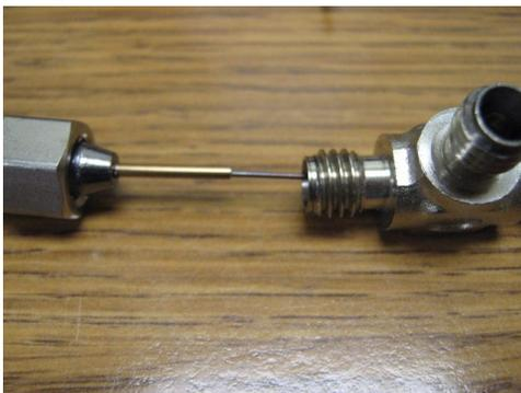
This is important because the sample will be split and to get a clean split the column must be inside the tube.
