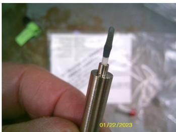
The hydrogen makeup supply can be connected to either restrictor tube. The NPD restrictor tube requires 10psi of H<sub>2</sub> pressure to get a flow of 2ml/minute.
