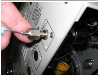
The EPC module is attached to the GC with two 5/64" hex head screws. Attached to the EPC solenoid is a pressure sensor. Both the sensor and the solenoid connect to the circuit board with 4 wire cables similar to those found on telephone handsets.
