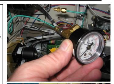
If a gauge is not available, you can calibrate the pressure using the gauge on the gas cylinder. Adjust the pressure on the gas cylinder so it is
