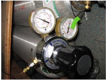
Verify that gas is arriving at the EPC bulkhead fitting by loosening the nut so you can hear the gas hissing out. If you can not hear the gas escaping then there may be a blockage between the gas cylinder and the GC.
