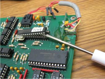
Replace it with the new chip. The part# of the new chip is 8600-1053. Cost as of Nov 2104 is \$110.
