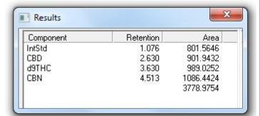
Notice how this is different than the External Standard Calibration curve where the number is the area of the CBD peak, not the ratio.
