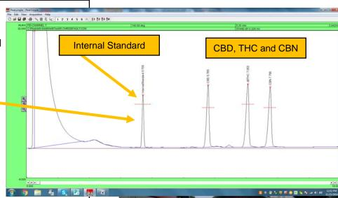
SRI suggests the Methyl stearate molecule ( CAS# 112-61-8 ) because its cheap, non-toxic and elutes in a convenient place in the chromatogram just before CBD. Its oil from the palm tree and used widely in lipstick, cosmetics and hand lotion.
