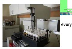
The "Internal Standard" method of calibration eliminates most of this problem.
