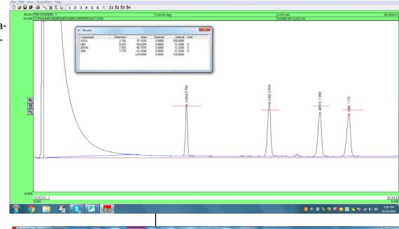
Here is the same exact data calibrated using the External Standard method. Both the peak areas and concentrations are identical.
