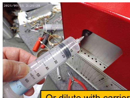
Or dilute with carrier gas by using the GC's injection port to fill the syringe.
