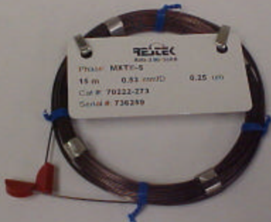
The 26 ga. Syringe needle fits inside the .53mm column to accomplish a cool on-column injection as specified in the method.
