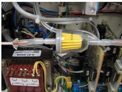
Adjust the filter and tubing so it does not touch any other parts inside the GC.
