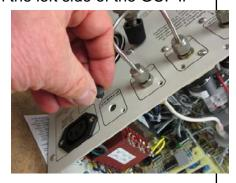
Tighten the power jack in the hole using the nut.
